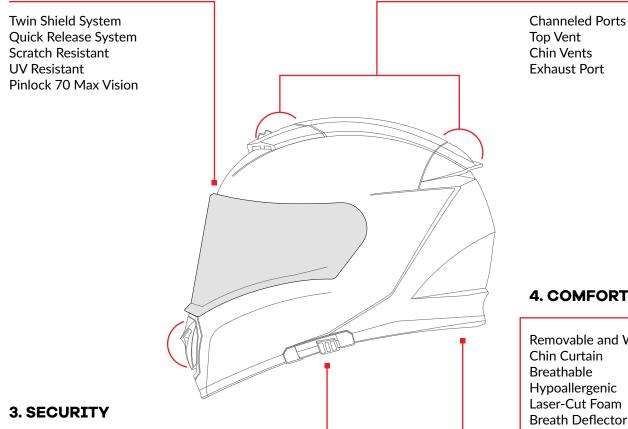
Steel Quick Release Buckle **Emergency Release System** Reinforced Chin Strap Metal Security Plate Reflective Safety Patch Multi-Density EPS Neck Roll
